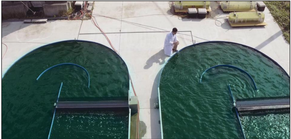
Figure 3. Euglena algae cultivation in raceway ponds for biodiesel production in Japan 2019. Image source: https://www.japan.go.jp/technology/innovation/fuelingjet.html
