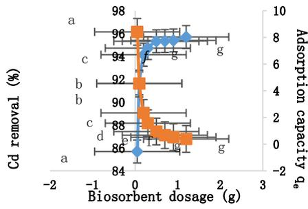
Figure 2 The effect of dosage of biosorbent on biosorption of Cd [pH = 5;  $C_o = 5 \text{ mg/L}$ ;  $t = 180 \text{ minutes}$ ]
