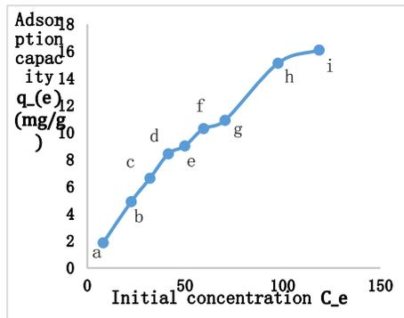
Figure 4. The effect of initial concentration on biosorption of Cd [pH = 5; 0.4 g biomass;  $t = 45 \text{ minutes}$ ]
