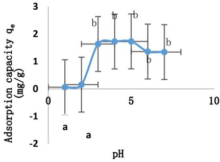
Figure 1. The effect of pH on biosorption of Cd [0.3 g biomass;  $C_o = 5 \text{ mg/L}$ ;  $t = 180 \text{ minutes}$ ]
