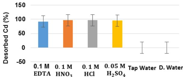
Figure 5. Desorption experiment [pH = 5; 0.4 g biomass;  $C_o = 8 \text{ mg/L}$ ;  $t = 45 \text{ minutes}$ ]
