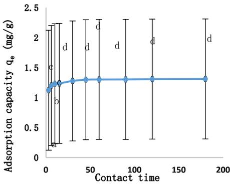
Figure 3. The effect of contact time on biosorption of Cd [pH = 5; 0.4 g biomass;  $C_o = 5 \text{ mg/L}$ ]
